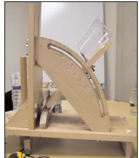
Figure 1: Device for controlling angle of the pour
