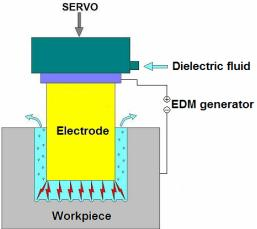
There are different variations of EDM processes including die sink EDM, wire EDM and EDM fast hole drilling. The main difference between fast hole drilling and other processes lies in the use of a high pressure (70 – 100 bar) dielectric pump. The combination of the high pressure dielectric fluid, the rotation of the tubular electrode and the high electrode feed rate (controlled by a fast response servo) make it possible to produce holes at a very *fast* rate.
