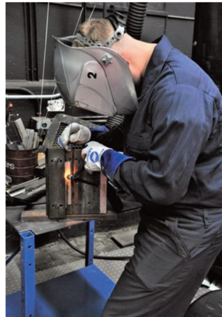
Figure 2: An Aviation Structural Mechanic Making a Practice Weld (Naval Air Systems Command 2018)
