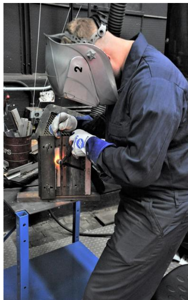
Figure 2: An Aviation Structural Mechanic Making a Practice Weld (Naval Air Systems Command 2018)
