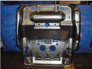
Seat pan – showing location of the 4 weld nuts
