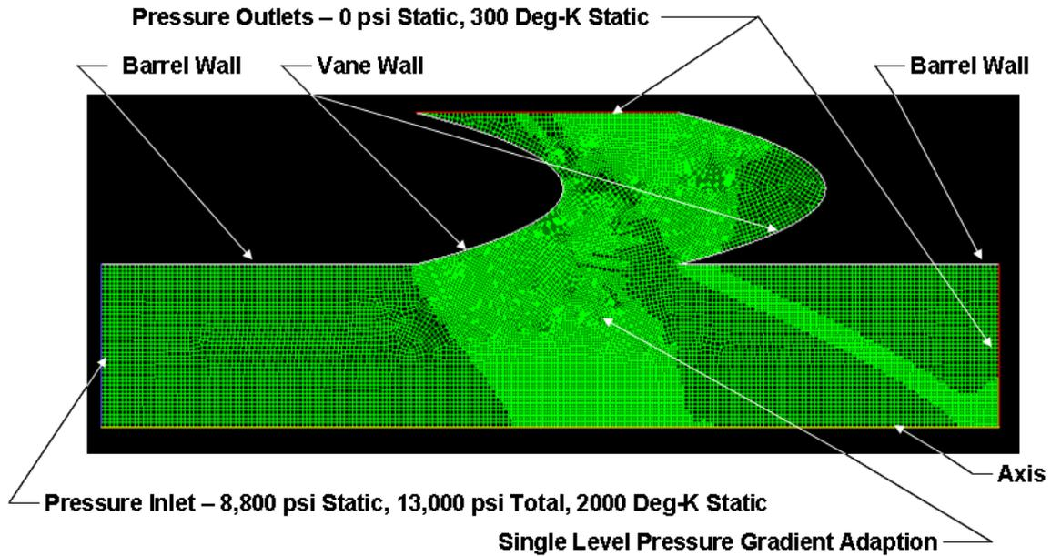
**Figure 3: CFD grid and boundary conditions**
