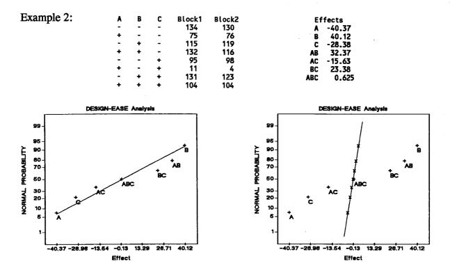
Based on the normal probability plot of the effects we might conclude all the effects are null. Augmenting the plot with the pure error effects clearly indicates 6 large effects. As in the previous example, ABC is the only null effect.
