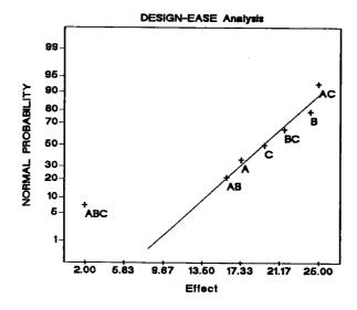
Based on this plot it looks like there is an ABC effect. But let's incorporate the pure error information on the normal probability plot. The sum of squares pure error is 263.00 with 7 degrees of freedom. The mean square pure error (263/7 = 37.57) estimates  $\sigma^2$ . Note that standard error for each effect is:
