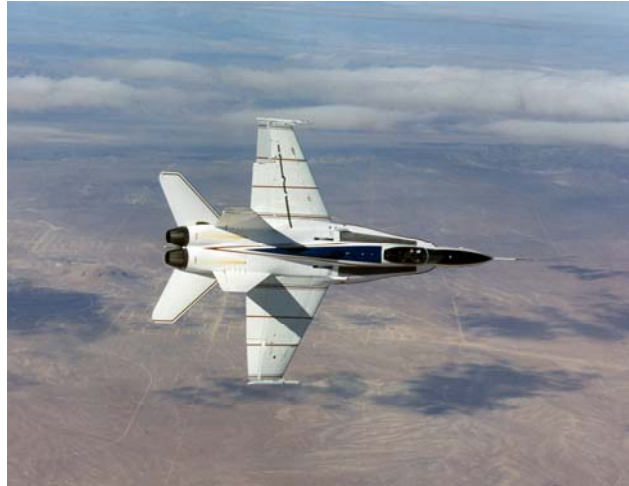
Figure 10-5: NASA's Active Aeroelastic Wing (AAW) F/A-18A research aircraft
